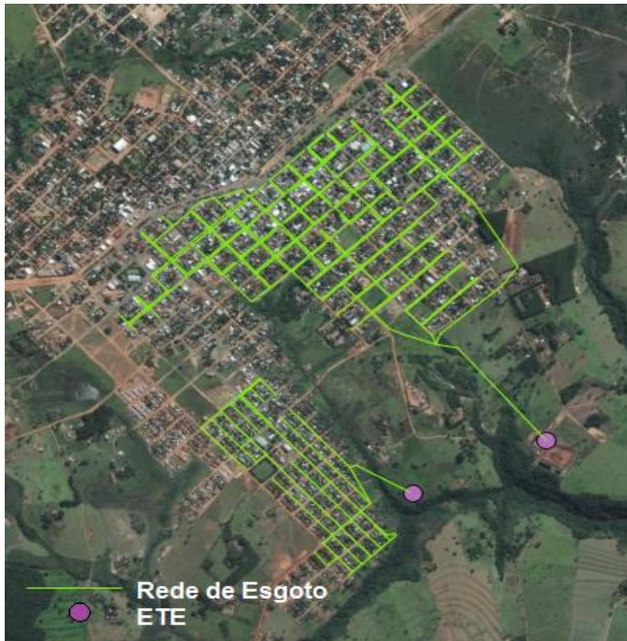
FIGURA 5: COBERTURA DA REDE COLETORA DE ESGOTO DE CORONEL SAPUCAIA.
